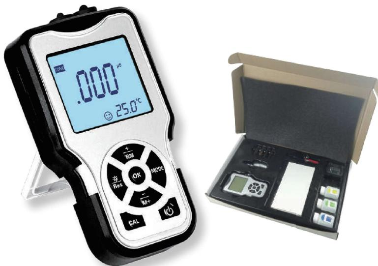
Measure conductivity, TDS, salinity, resistivity, dissolved oxygen and temperature of water solutions and very cost effective.
